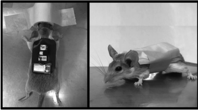
Fig. 5 NIC-Kidney Device adhered to the centre of the back. Spiny mouse with the NIC-Kidney Device and battery adhered in a linear fashion across the back on the rodent.
