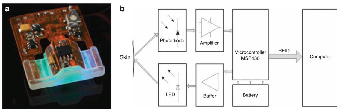
**Figure 1 | New device.** Optical part of the new device for transcutaneous measurement (a) and a schematic drawing of its building blocks (b). LED, light-emitting diode; RFID, radio-frequency identification.
