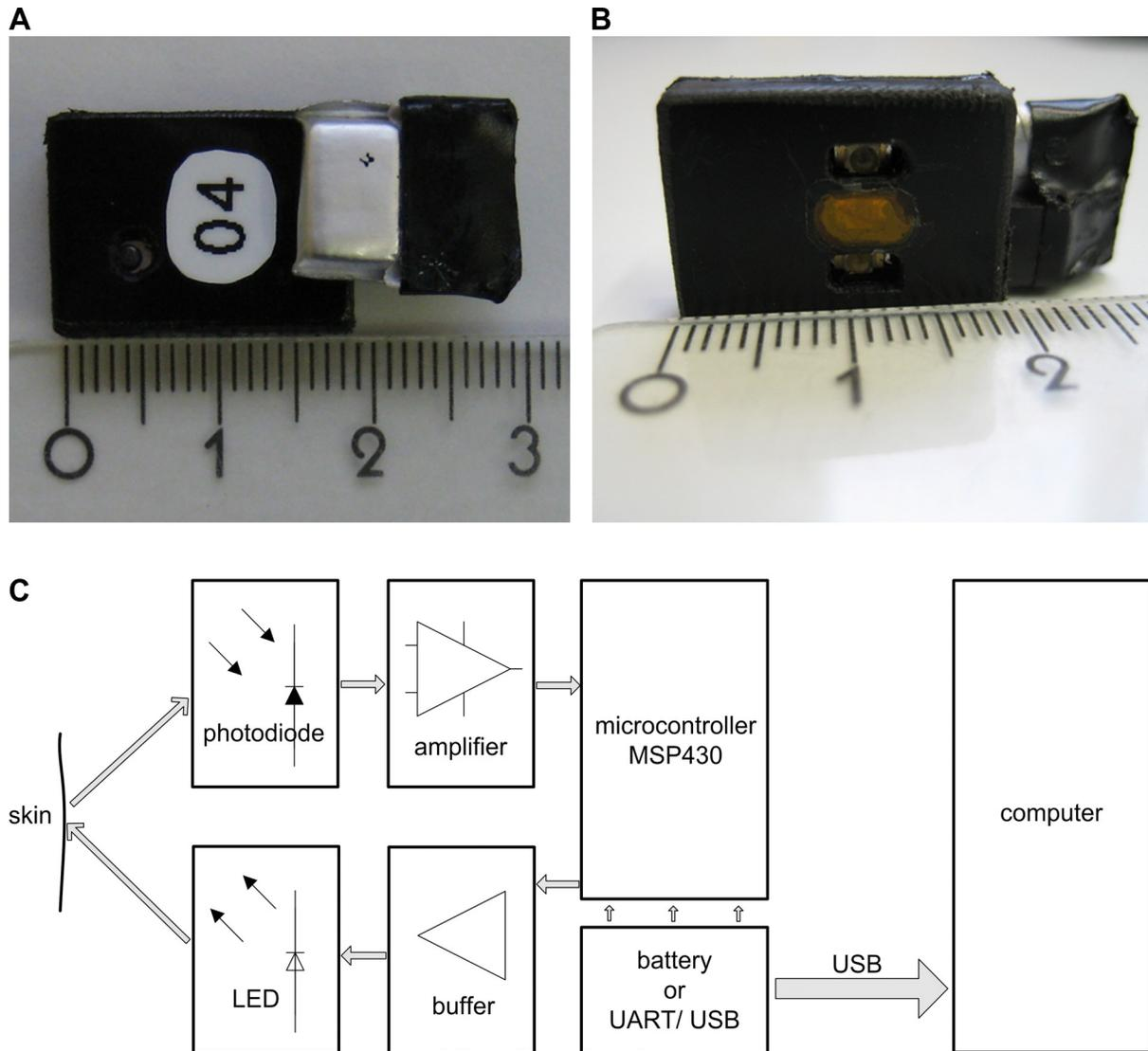
Fig. 1. Top (A) and bottom (B) view of the miniaturized device with battery for transcutaneous measurement (ruler in cm). C: schematic drawing of its building blocks.
