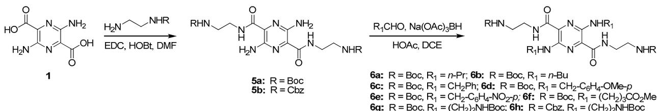
**Scheme 2.** Synthesis of small molecule pyrazine scaffolds by reductive amination.
