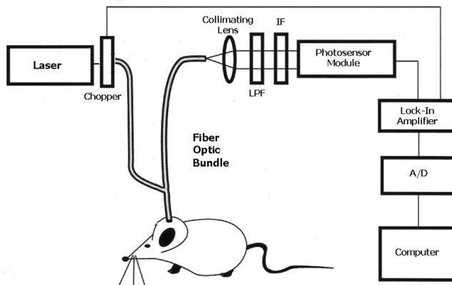
**Figure 1.** Apparatus for non-invasive *in vivo* detection of fluorescence.
