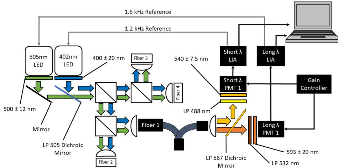
Figure 3: Transdermal fluorescence detection system schematic illustrating the illumination system and one of four identical detection channels.
